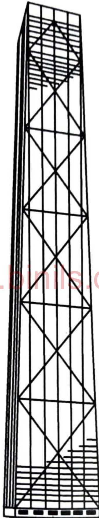
Fig. 2.3.16 : Steel-braced tube structure
