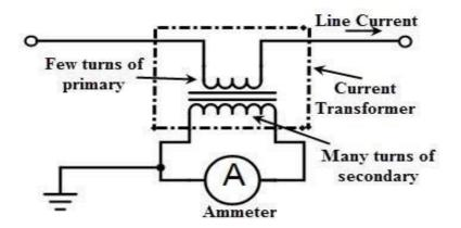
Primary of C.T. is having very few turns. Sometimes bar primary is also used. Primary is connected in series with the power circuit. Therefore, sometimes it also called series transformer.
