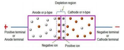
Cathode is the negatively charged electrode or conductor, which supplies free electrons to the p-n junction. In other words, cathode terminal or negative terminal is the source of free electrons, the negative charge carriers (free electrons) begins their journey at cathode terminal and travel through the diode and ends at anode terminal.
