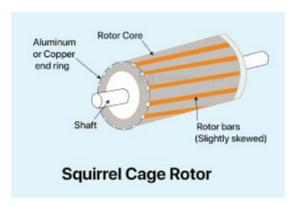
Most of the induction motors (upto 90%) are of squirrel cage type. **Squirrel cage type rotor** has very simple and almost indestructible construction. This type of rotor consists of a cylindrical laminated core, having parallel slots on it. These parallel slots carry rotor conductors. In this type of rotor, heavy bars of copper, aluminum or alloys are used as rotor conductors instead of wires. Rotor slots are slightly skewed to achieve following advantages -
