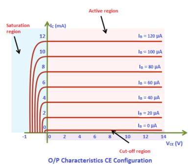
A curve is then drawn between output current  $\, I_C \,$  and output voltage  $\, V_{CE} \,$  at constant input current  $\, I_B \, (0 \, \mu A).$
