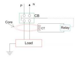
Single Phase Residual Current ELCB. The polarity of the phase winding and neutral winding on the core is so chosen that, in normal condition mmf of one winding opposes that of another.
