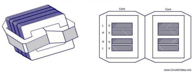
The coils are form-wound but are multi layer disc type usually wound in the form of pancakes. Paper is used to insulate the different layers of the multi-layer discs. The whole winding consists of discs stacked with insulation spaces between the coils. These insulation spaces form the horizontal cooling and insulating ducts. Such a transformer may have the shape of a simple rectangle or may also have a distributed form.
