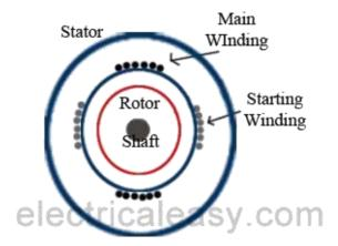
of three phase\_induction motor having squirrel cage rotor, except that the stator is wound for single phase supply. Stator is also provided with a 'starting winding' which is used only for starting purpose. This can be understood from the **schematic of single phase induction motor** at the left.
