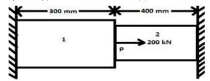
at point, P (ii) Stress in each element (iii) Reaction force
