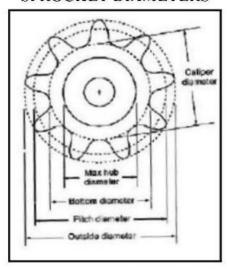
The equal piniter com diameter and pinitersity, Polytechnic & Schools (i) Pitch diameter =  $\frac{p}{\sin(\frac{180}{z})}$  Free PDF Study Materials
