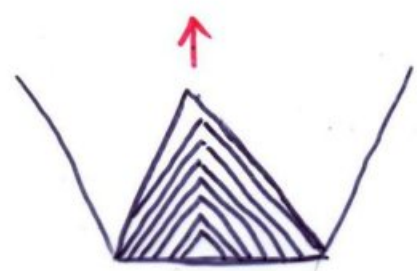
Applying Depth of cut \perp to the lathe axis
