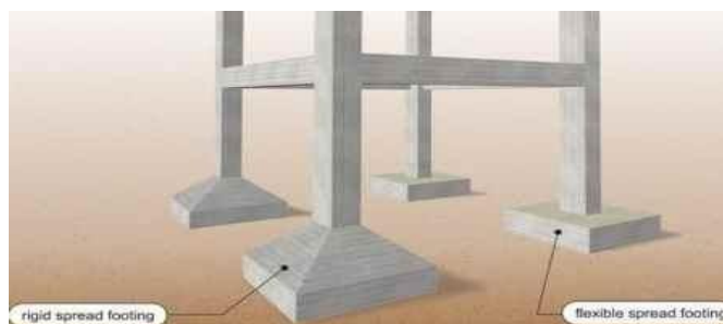
Fig 5: Flexible and Rigid Footings of a Structure
