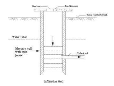
For the purpose of inspection of well, the manholes are provided in the top cover. The water filtrates through the bottom of such wells and as it has to pass through sand bed, it gets purified to some extent. The infiltration well in turn are connected by porous pipes to collecting sump called jackwell and there water is pumped to purification plant for treatment.
