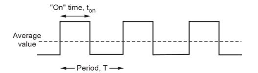
The average value can be extracted from the PWM stream with a low-pass filter. In this case, and as long as PWM frequency and values of R and C are appropriately choosen, Vout becomes an analog output.
