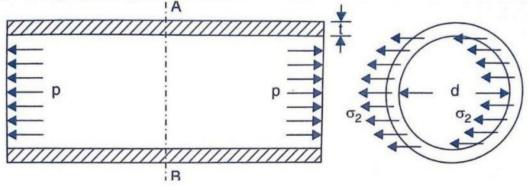
The longitudinal stress ( $\sigma_2$ ) developed in the material is obtained as:
