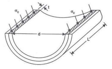
$\sigma_c$  = Compressive circumferential stress exerted by wire on cylinder
