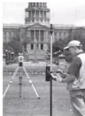
Robotic total station
