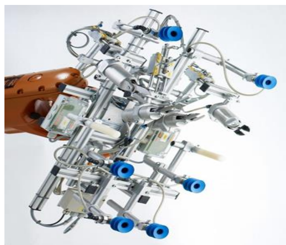
Robot end-of-arm tooling with slide-out nippers and part sensors for plastics injection molding. (Courtesy of ASS End of Arm Tooling, Inc.)
