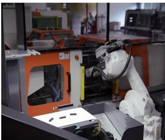
Six-axis articulated robot tends an injection molding machine producing plastic components for ear protectors. (Courtesy of ABB Robotics)
