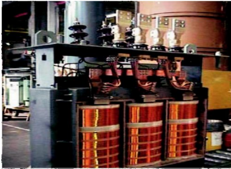
Figure 5.15 1600 kVA Amorphous Core Transformer
