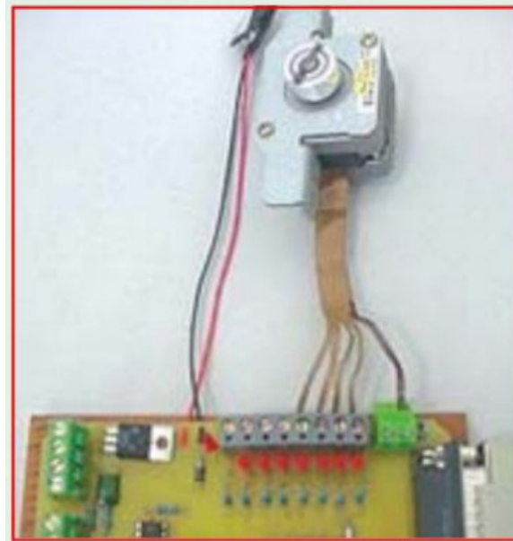
Connecting a stepper motor to the interface
