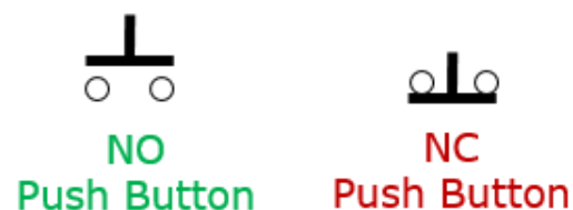
Figure 1.1 Symbol of Pushbutton
