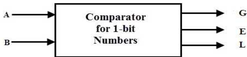
Fig 4.49 (a) Block diagram of single bit comparator
