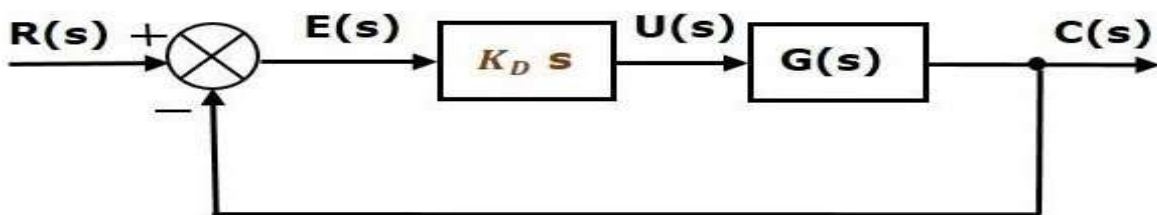
Figure 2.5.2: block diagram of derivative controller
