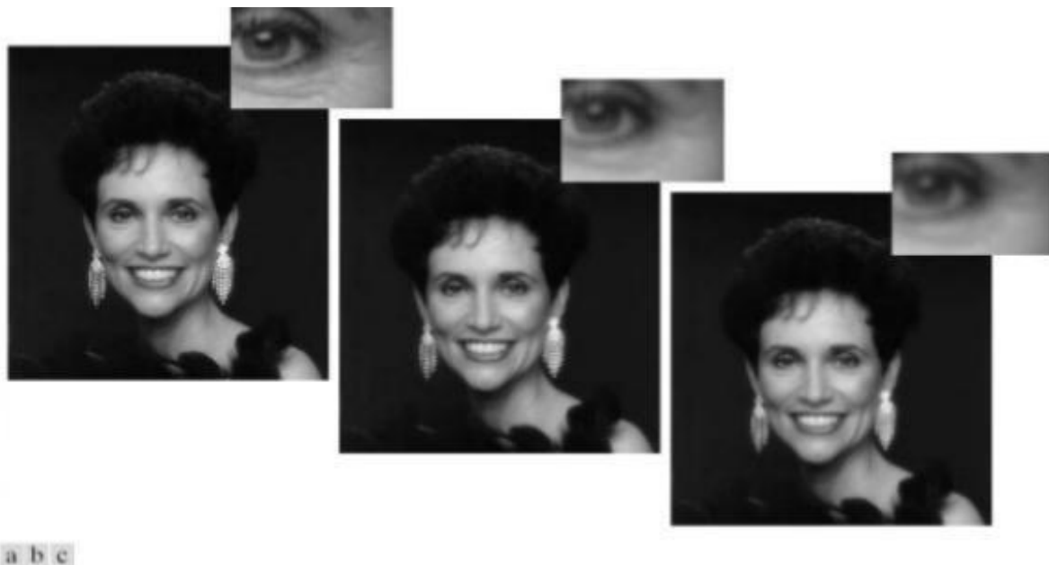
Fig. 2.2.7(a) Original image (784x 732 pixels). (b) Result of filtering using a GLPF with D_0 = 100 . (c) Result of filtering using a GLPF with D_0 = 80 . Note the reduction in fine skin lines in the magnified sections in (b) and (c).
