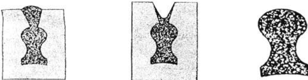
Fig. 4.5.1- Solid slip casting
