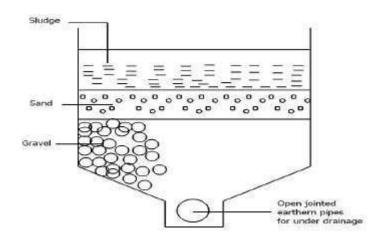
A sludge drying bed usually consists of a bottom layer of gravel of uniform size over which is laid a bed of clean sand. Open jointed tile under drains are laid in the gravel layer to provide positive drainage as the liquid passes through the sand and gravel.
