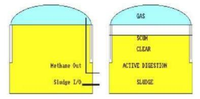
The gas is collected in a steel gas holder placed at the top of digestion tank; the average composition of biogas is as follows Methane-55%, Carbondioxide 35%, Hydrogen 7.4% and Nitrogen 2.6%. Biogas improves local sanitation and health. The main objective during AD is to recover methane gas which could serve as combustible in various area of the economy, including generation of electricity, heating, and in kitchen.
