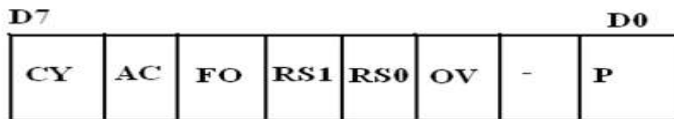
Figure 3.1.2 Program Status Word of 8051 Microcontroller
