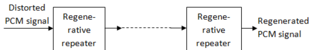
Figure 5.7.4: PCM Transmission path
