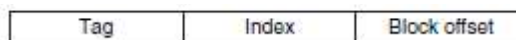
Figure: Three portions of an address in a set-associative or direct-mapped cache.
