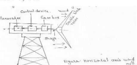
A propeller consisting of two or three blades (with an aerofoil section) and capable of running at the high speeds is likely to be the most efficient. Present technology has been able to build systems with 60m long blades, a lowers as high as 305m. A large tower system, to support many small rotor – generator units, can also be built.
