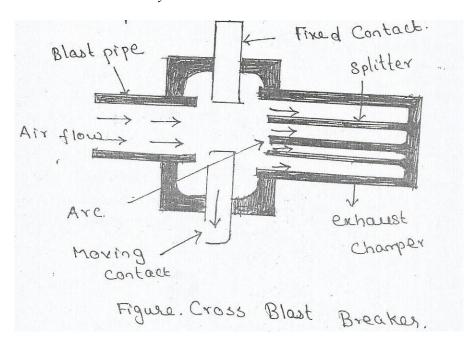
In this system the blast pipe is fixed in perpendicular to the movement of moving contact in the arcing chamber and on the opposite side of arcing chamber one exhaust chamber is also fitted at the same alignment of blast pipe, so that the air comes from blast pipe can straightly enter into exhaust chamber through the contact gap of the breaker.
