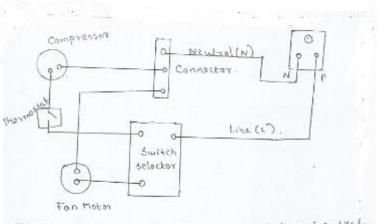
Figure : Electric Circuit diagram of window an anditioner
