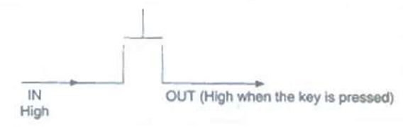
Fig 3.36: Basic keyboard operation – single key
