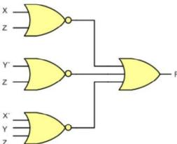
It can also be implemented using **OR-NAND** circuit as it is equivalent to NOR-OR circuit as shown in the figure.
